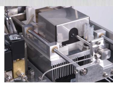
The electrical cooling of the sorbent trap, reaching -40 °C, offers advantages to almost every application, allowing to work without cryogenic liquids to retain very volatile compounds and to avoid the risk of ice formation. Additionally, the high temperature desorption capacity permits the extraction of analytes with volatility equivalent to that of n-C44 hydrocarbons.
