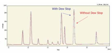
"Dew Stop" removes water maintaining the recovery of Chlorinated Hydrocarbons unaffected.
